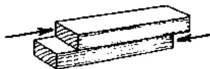
Horizontal shear produces a tendency for wood cells to separate and slide longitudinally. It is normally the controlling type of shear for wood members.
