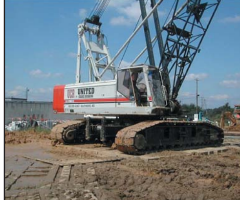
emtek mats makes poor soil conditions workable at a construction site.
