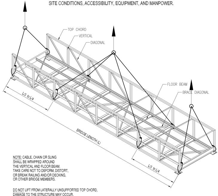
THE BRIDGE STRUCTURES ARE DESIGNED TO BE LIFTED FROM EITHER THE APPROXIMATE 1/4 TO 1/3 POINTS OR FROM THE BEARING LOCATIONS. BRIDGE STRUCTURES ARE NOT DESIGNED FOR LAUNCHING STRESSES.
