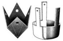
The trend toward heavier hammers and heavier design loading may mean that timber will be subjected to damaging blows when the pile reaches obstructions or end bearing. As a result, timber piles can be protected by a metal boot or point. The point shown in the picture covers the entire pile tip without the need for trimming the pile tip. Also shown is another type of point protection attachment, however requires minor trimming of the pile tip.
